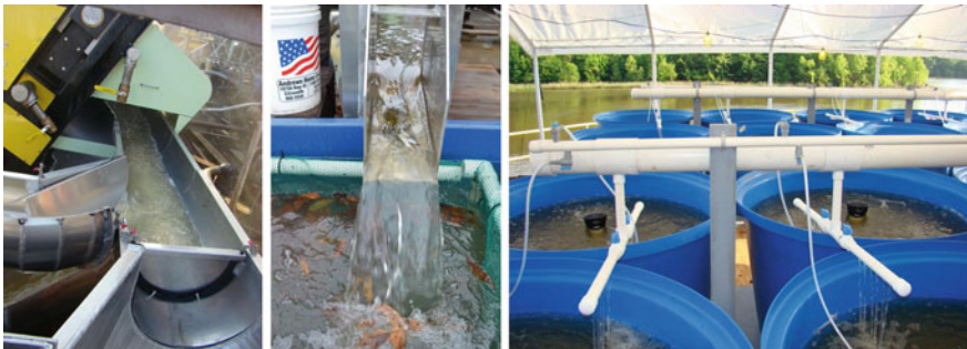
Fig. 4.3 Impingement survival sampling study. Impinged organisms are diverted from the screen's fish return trough ( left ) to a collection net ( middle ). Collected organisms are transferred to a holding facility ( right ) where they are held in flow-through tanks to assess latent impingement mortality. (Images courtesy Alabama Power Company)
