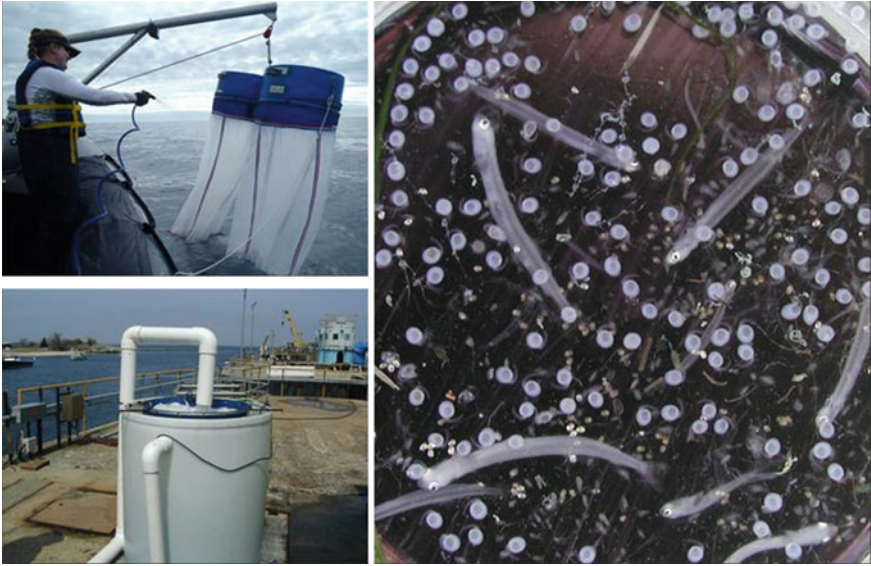
Fig. 4.5 Entrainment sampling equipment. Bongo plankton nets for collecting ichthyoplankton samples upstream of the intake structure ( top left ); barrel sampler with integral plankton net for collecting pumped samples from within intake structure ( bottom left ; image courtesy ASA Analysis and Communication, Inc.); and fish eggs and larvae collected during entrainment sampling studies
