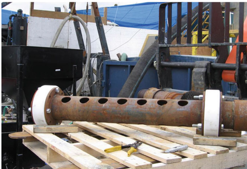
Fig. 13.22 Air lift swab used for initial development
