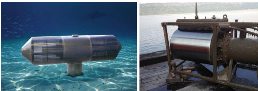
Fig. 4.8 Cylindrical wedgewire screen designs. Bilfinger Water Technologies screen with Hydroburst backwash cleaning system ( left ) and Intake Screens, Inc. screen with rotating, brush-cleaned screen drums (0.5-mm slot width) ( right )
