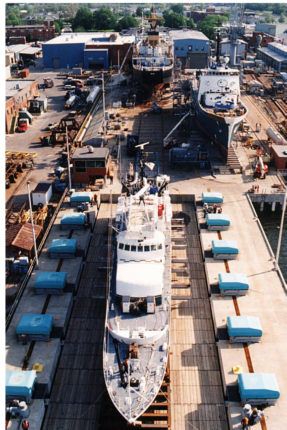
Figure 5: Single Level Transfer at US Coastguard
