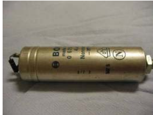
PCB in capacitors for light fixtures and one phase motors
