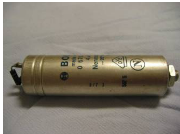
Figure 2: Typical capacitor that may contain PCB
