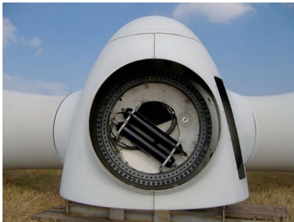
Fig. 2.5 Hydraulic pitch system. (Courtesy of Wikimedia commons (KarleHorn 2010). This file is licensed under the Creative Commons Attribution-Share Alike 3.0 Unported license)
