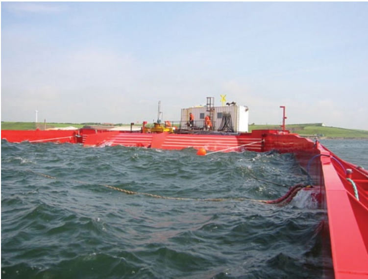
Fig. 5.3 Wave Dragon WEC seen from its reflector. (Courtesy of Erik Friis-Madsen (Friis-Madsen 2010). This file is licensed under the creative commons attribution 3.0 unported license)
