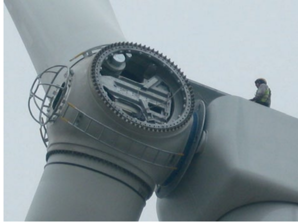
Fig. 2.3 Hub. (Courtesy of Paul Anderson (Anderson, Hub of Turbine No 23— geograph.org.uk —837248.jpg, 2011a). This file is licensed under the Creative Commons Attribution-Share Alike 2.0 Generic license)
