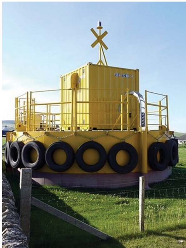
Fig. 5.13 Test buoy for EMEC wave scale test site, scapa flow. (Curtis 2012, © Copyright Andrew Curtis and licensed for reuse under this Creative Commons Licence)
