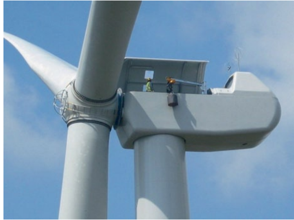
Fig. 2.2 Nacelle of a wind turbine. (Courtesy of Paul Anderson (Anderson, Nacelle of Turbine Tower No 26— geograph.org.uk —824692.jpg, 2011b). This file is licensed under the Creative Commons Attribution-Share Alike 2.0 Generic license)
