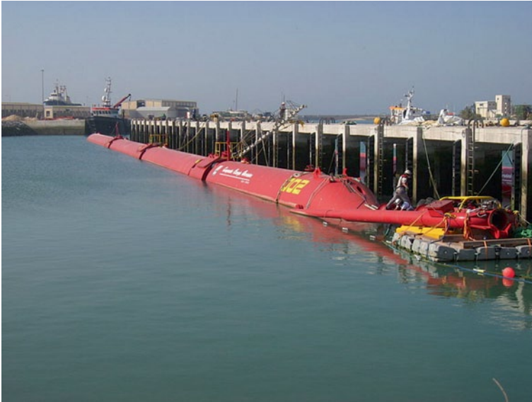
Fig. 5.7 Pelamis wave energy converter. (Courtesy of Guido Grassow (Grassow 2007). The file is licensed under creative commons attribution-share alike 3.0 unported license)
