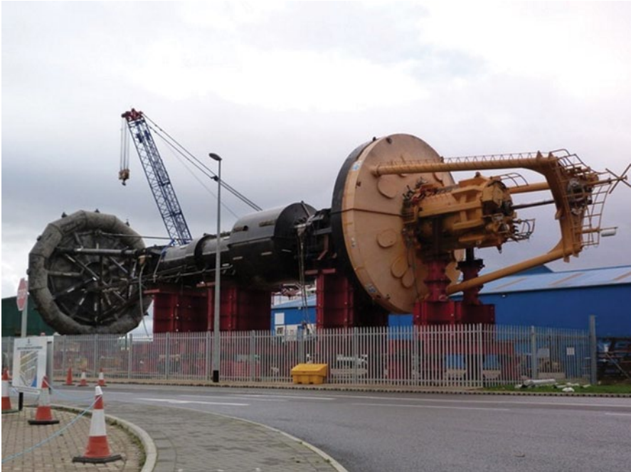
Fig. 5.17 PowerBuoy wave energy converter. (Duckworth 2011. © Copyright Sylvia Duckworth and licensed for reuse under this Creative Commons Licence)
