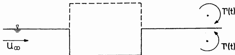
Fig. 6.14. Simple vortex system with an image flow above the free-surface so that the rigid free-surface condition is satisfied.
