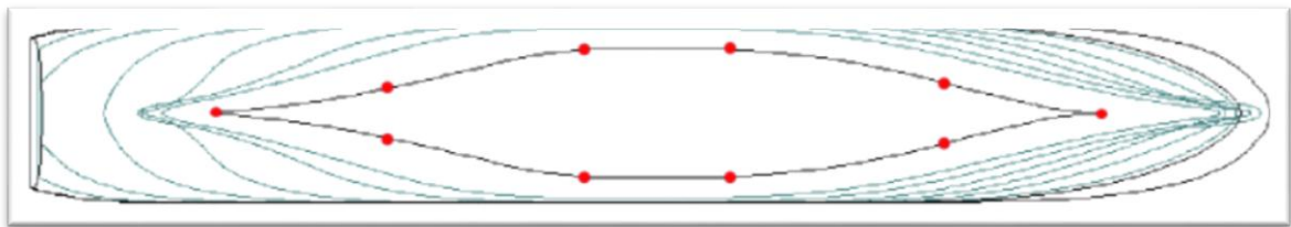
Figure 2.10: Typical critical point locations on ships keel [Vantorre et al., 2008]
