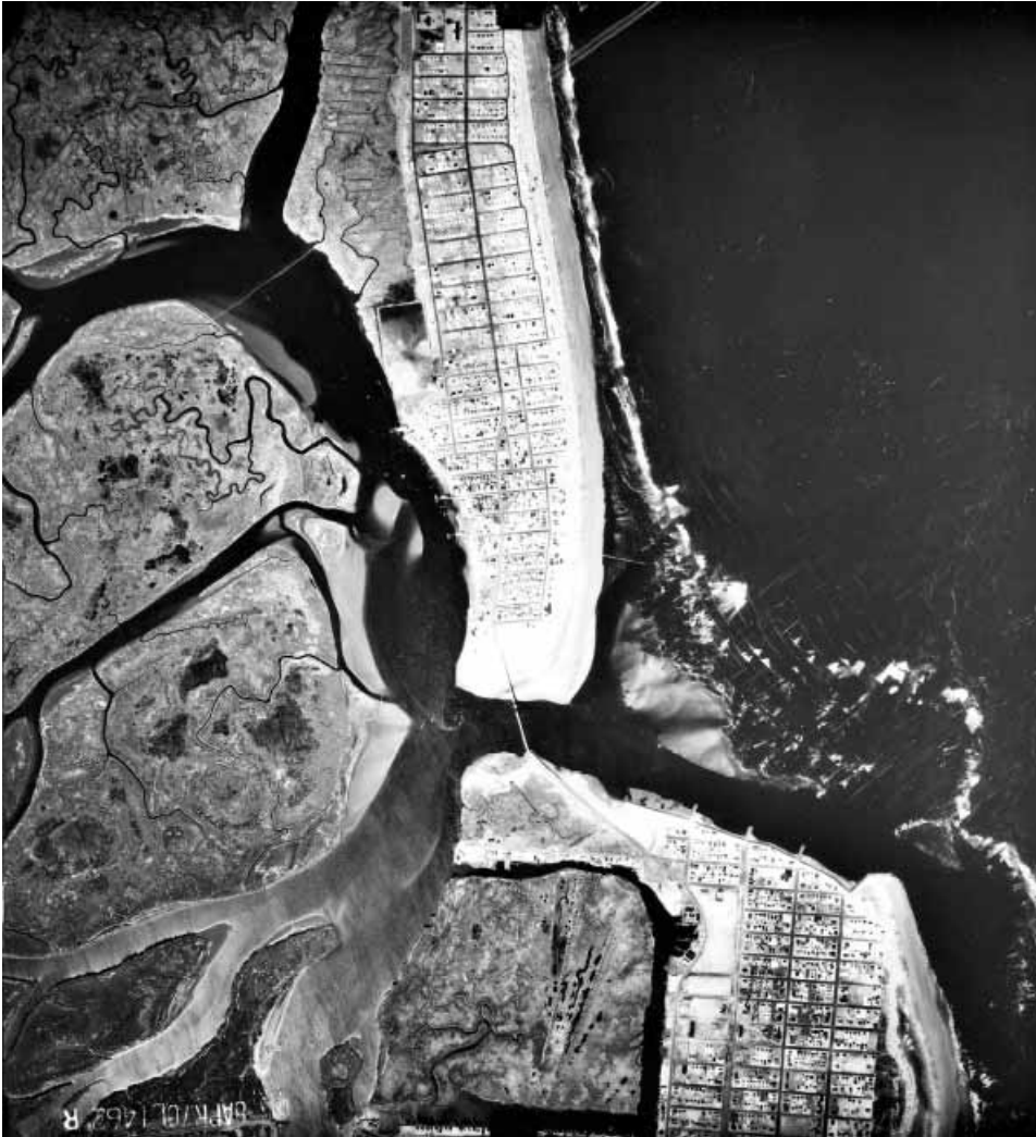
Figure 3.21 Townsends Inlet, New Jersey. The net littoral drift is from north (top) to south.
