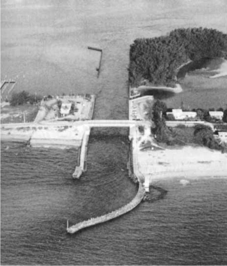
Figure 13.19 South Lake Worth Inlet, Florida. Note the sand transfer plant on the north jetty (from Yeend and Hatheway 1988).
