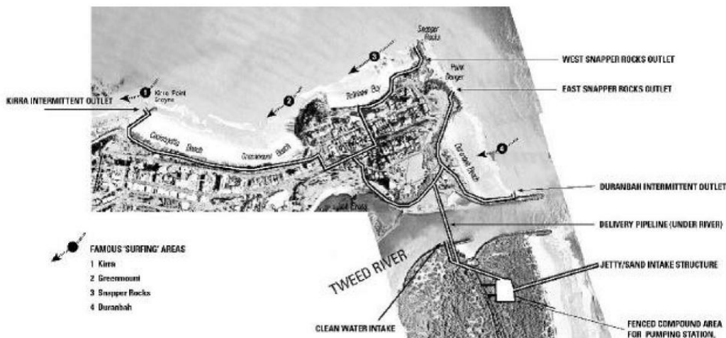
Figure 8-12. Tweed River sand bypassing scheme
